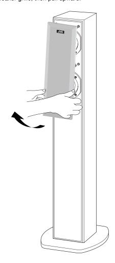
To attach the speaker grille, put the projections of the speaker into the holes of the speaker grille.
